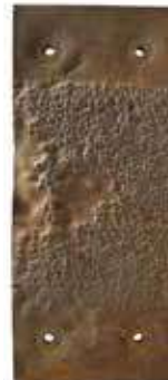
Used apron plate with minimal wear after 74,000 tons
